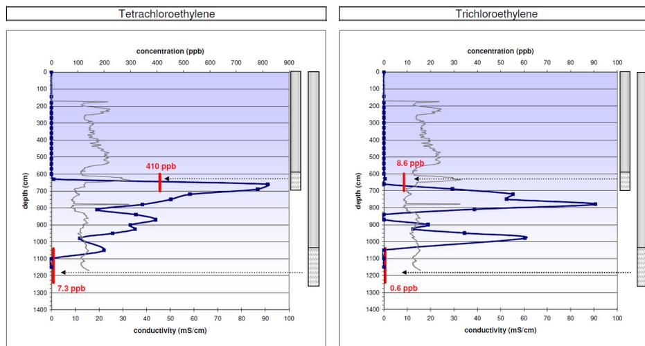
**Fig. 3: EnISSA measurements for PCE and TCE compared to results obtained with a sampling well.**
