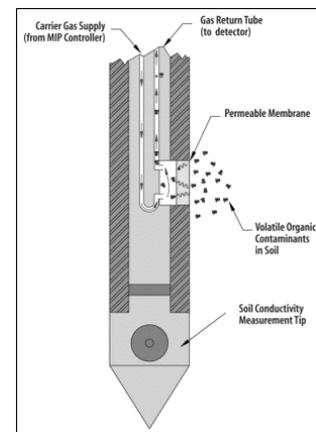
**Fig. 1: Membrane Interface Probe (MIP)**
